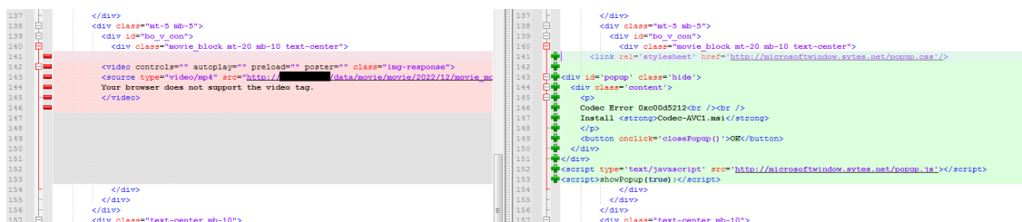
Figure 3. A comparison of the webpage content between the original page (left) and the page with the injected script (right)
