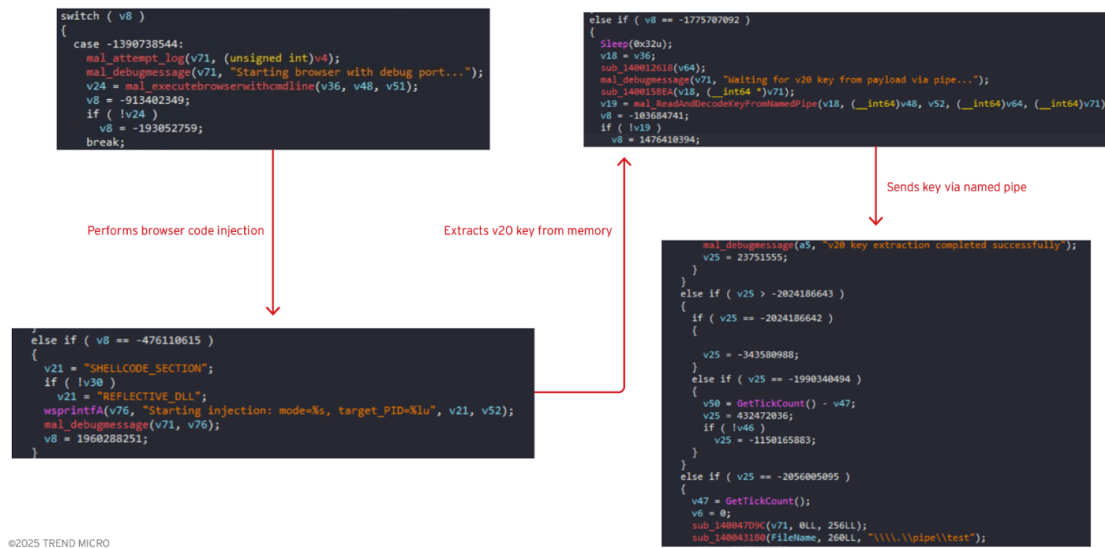
Figure 5. Encryption keys stolen from browser memory are sent back to malware process via named pipes
