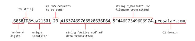
Figure 4 Subdomain that ALMA Communicator attempts to resolve to transmit data to its C2 server
