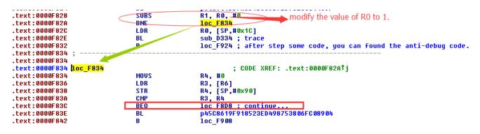
Figure 17. How to bypass the anti-debug code
