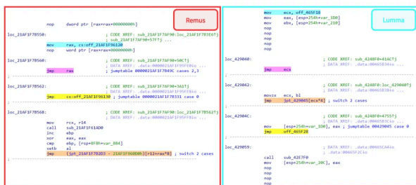
Figure 28: Randomly selected disassembly code from Remus (left) and Lumma (right) highlighting the different forms of the discussed indirect control flow obfuscation.
