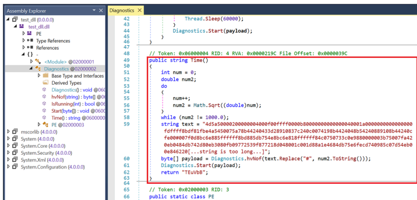
Figure 12: dnSpy screenshot showing the payload that will be launched in memory
