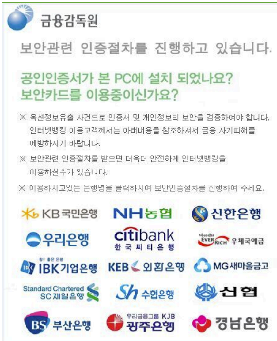
Figure 13: Message displayed when user of infected client visits a domain listed in modified Hosts file
