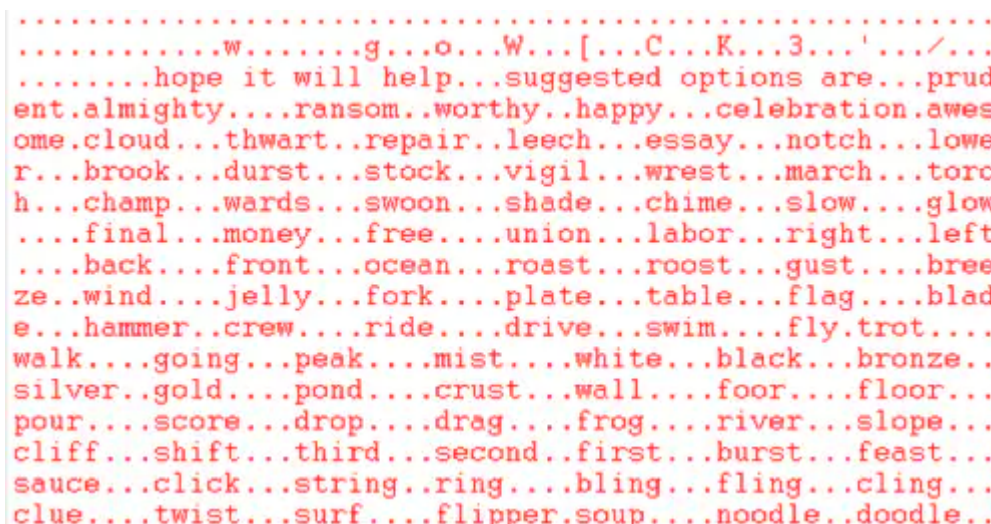
Figure 3 – A memory dump from a CONFUCIUS_A sample showing the lookup table used by the malware, the table is truncated for presentation purposes.
