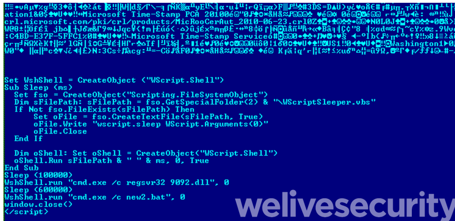
Figure 7. Example of a script appended to the PE file signature section
