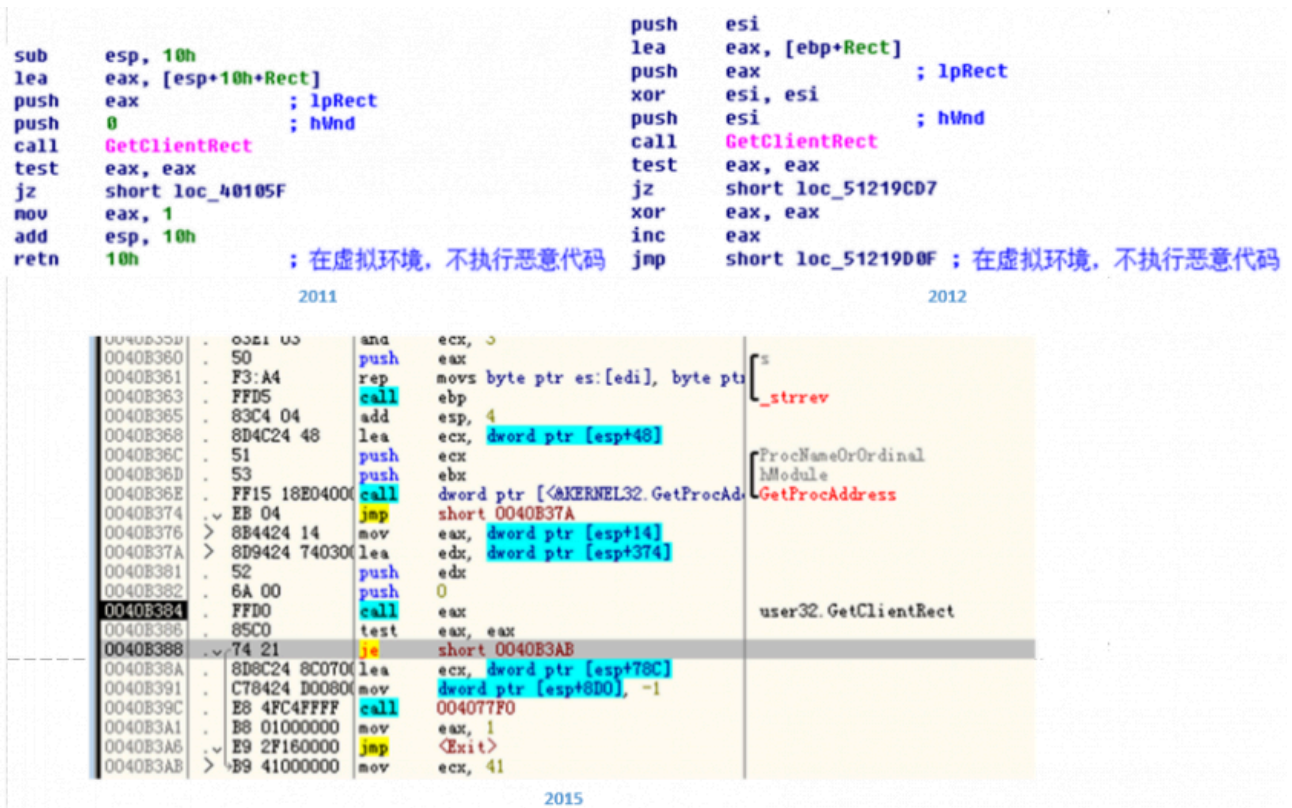
Figure 20: Another way to evade detection systems is to pass the wrong parameter to 'GetClientRect'.
