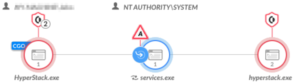
Figure 21. HyperStack creates a service for persistence shown in Cortex XDR in detect mode.
