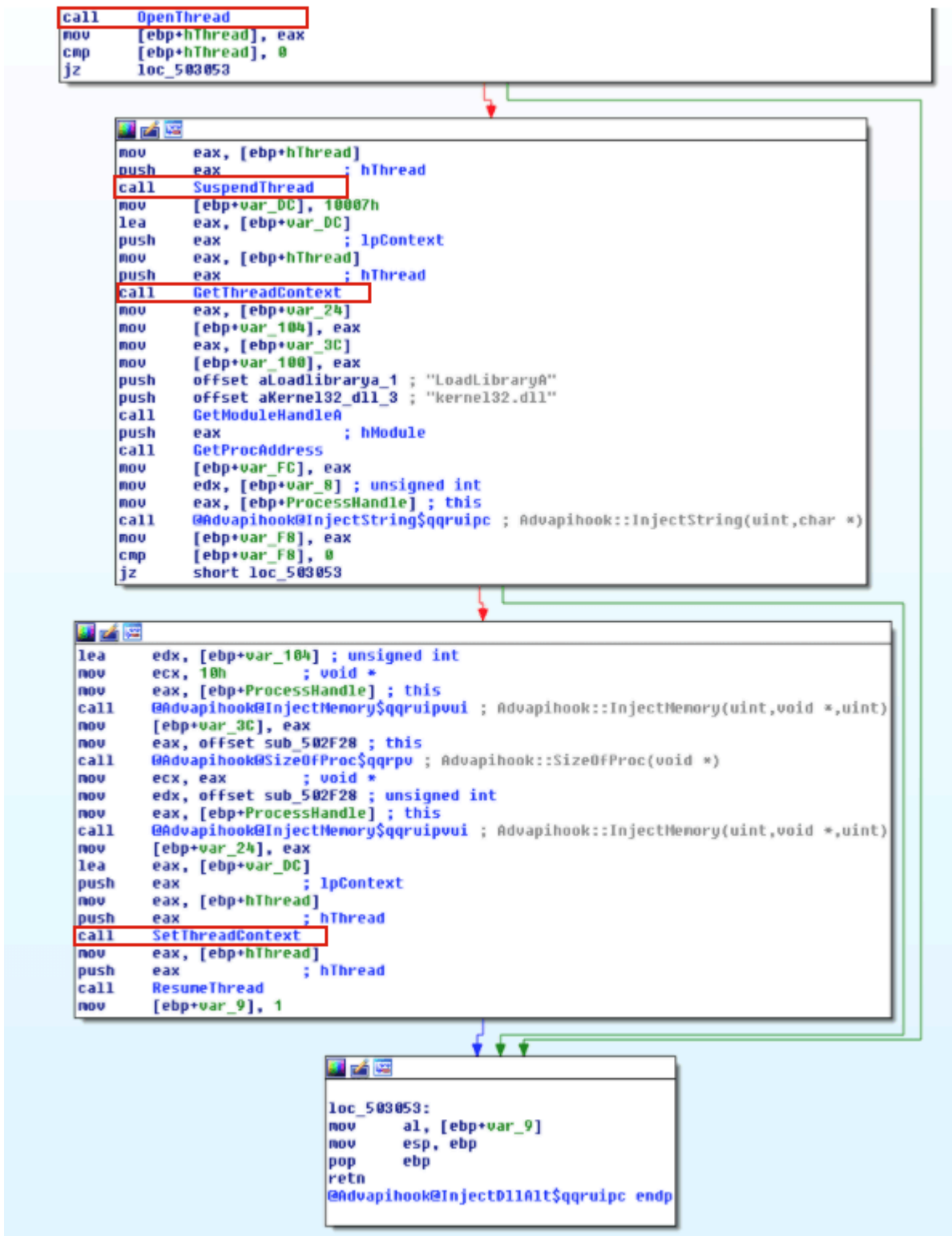
Figure 4: A generic trojan is performing thread execution hijacking Sha256: 787cbc8a6d1bc58ea169e51e1ad029a637f22560660cc129ab8a099a745bd50e
