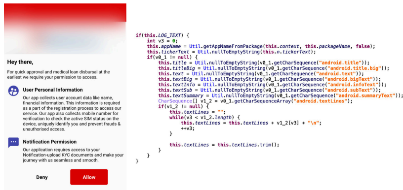
Figure 15. Request notification permission as seen by the user (left), and the code to parse the notification (right)
