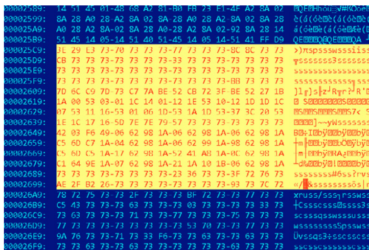
Figure 45: A single XOR byte key is used to encrypt the executable file and is embedded using steganography at the offset 0x25c9.
