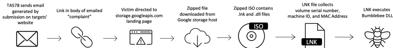
Figure 11: "Contact Form" attack chain leading to Bumblebee
