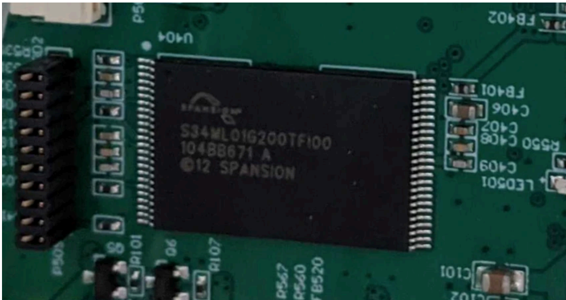
The NAND Flash chip used by the Contec CMS8000.
