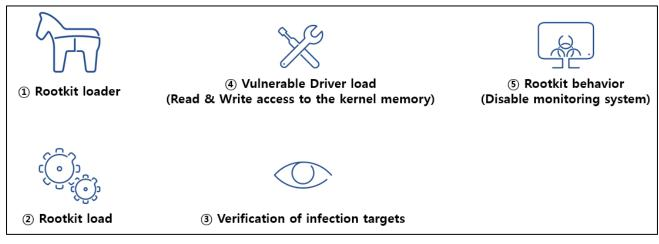
Figure 4. Rootkit execution flow ( $1 \sim 5$ )
