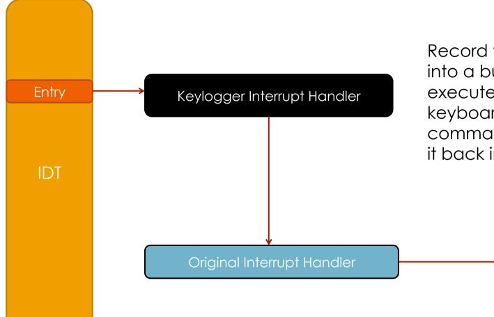
Record the keystroke into a buffer and execute the special keyboard controller command for putting it back into place
