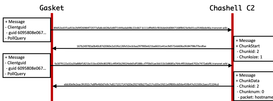
Figure 3. Example DNS request and response flow of Chashell.
