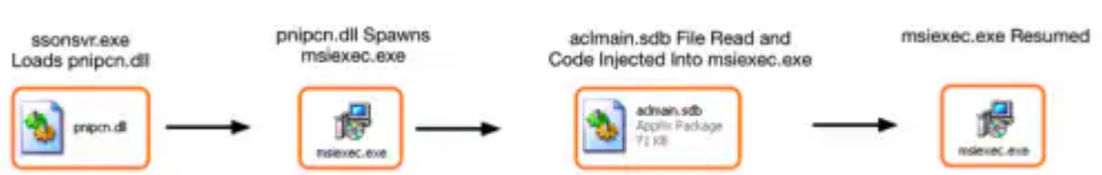
Figure 6 Sideload execution flow
