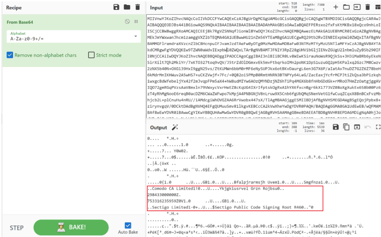
Figure 10 - Extracted malformed digital signature from JavaScript QakBot Loader
