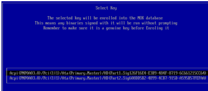
MokManager, a part of shim bootloader used to enroll Machine Owner Key (MOK) to UEFI system
