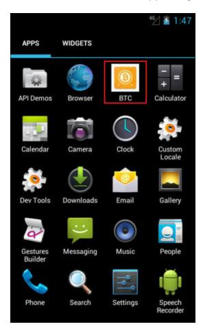
Once the Trojan is launched on an infected device, it displays a fake error message and continues to operate in hidden mode. The Trojan hides its icon from the list of applications on the Android home screen. From now on, the malware can be found in the apps management section of the system preferences only. Both modifications of **Android.Clipper** are then launched automatically every time an infected smartphone or tablet is turned on.
