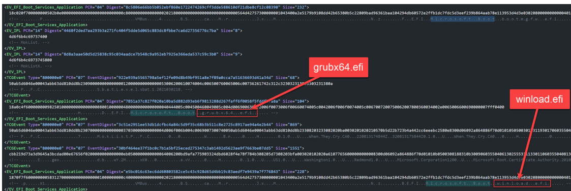
Figure 9: BlackLotus components visible in MeasuredBoot logs after parsing to XML
