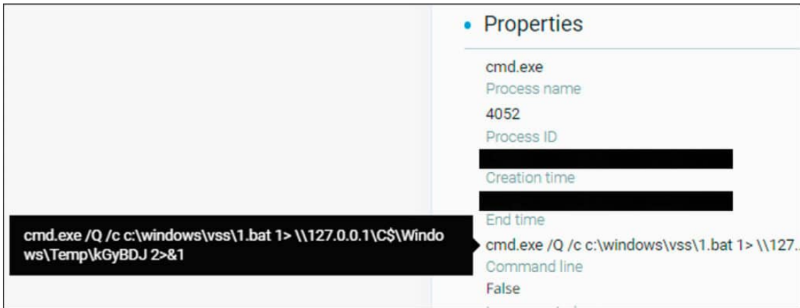
Snippet showcasing the WMIExec command being executed on a victim machine with batch script '1.bat'
