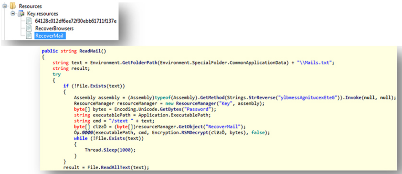
Figure 3: The Nirsoft utilities are stored in encrypted form and extracted and executed on the fly.
