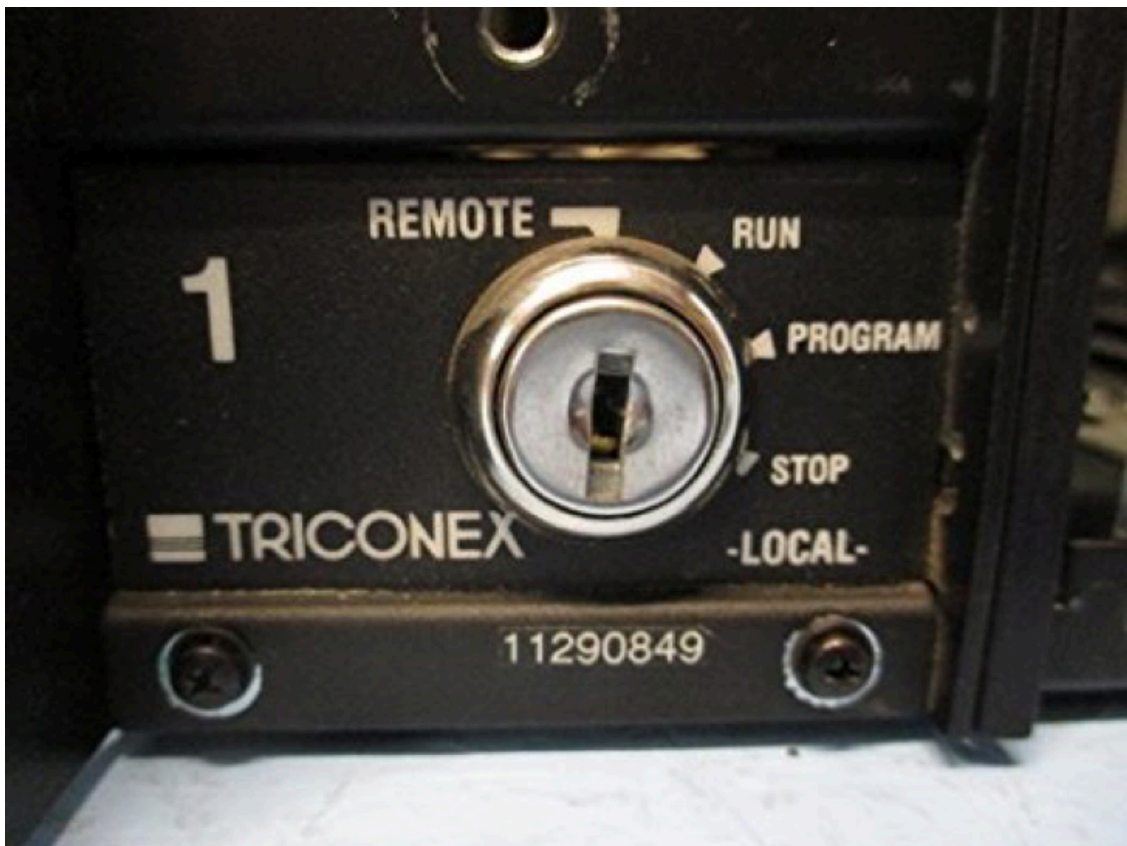
Figure 3: Triconex Key Switch ( source )
