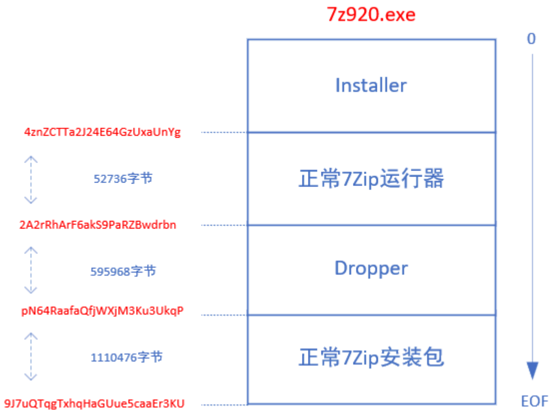
Figure 2-2 Schematic diagram of decoy installation package
