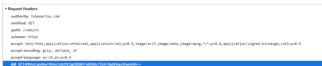
Figure 30. An example of the added dd header.
