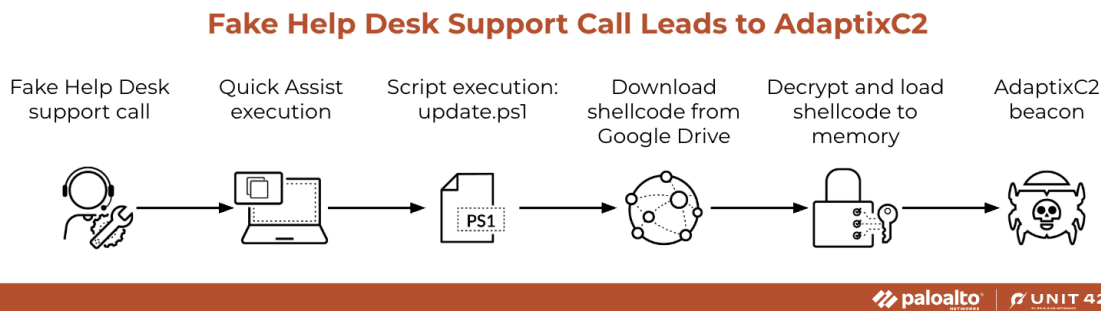
Figure 3. Attack vector of AdaptixC2 installation on victim machine. Source: Unit 42 X post .
