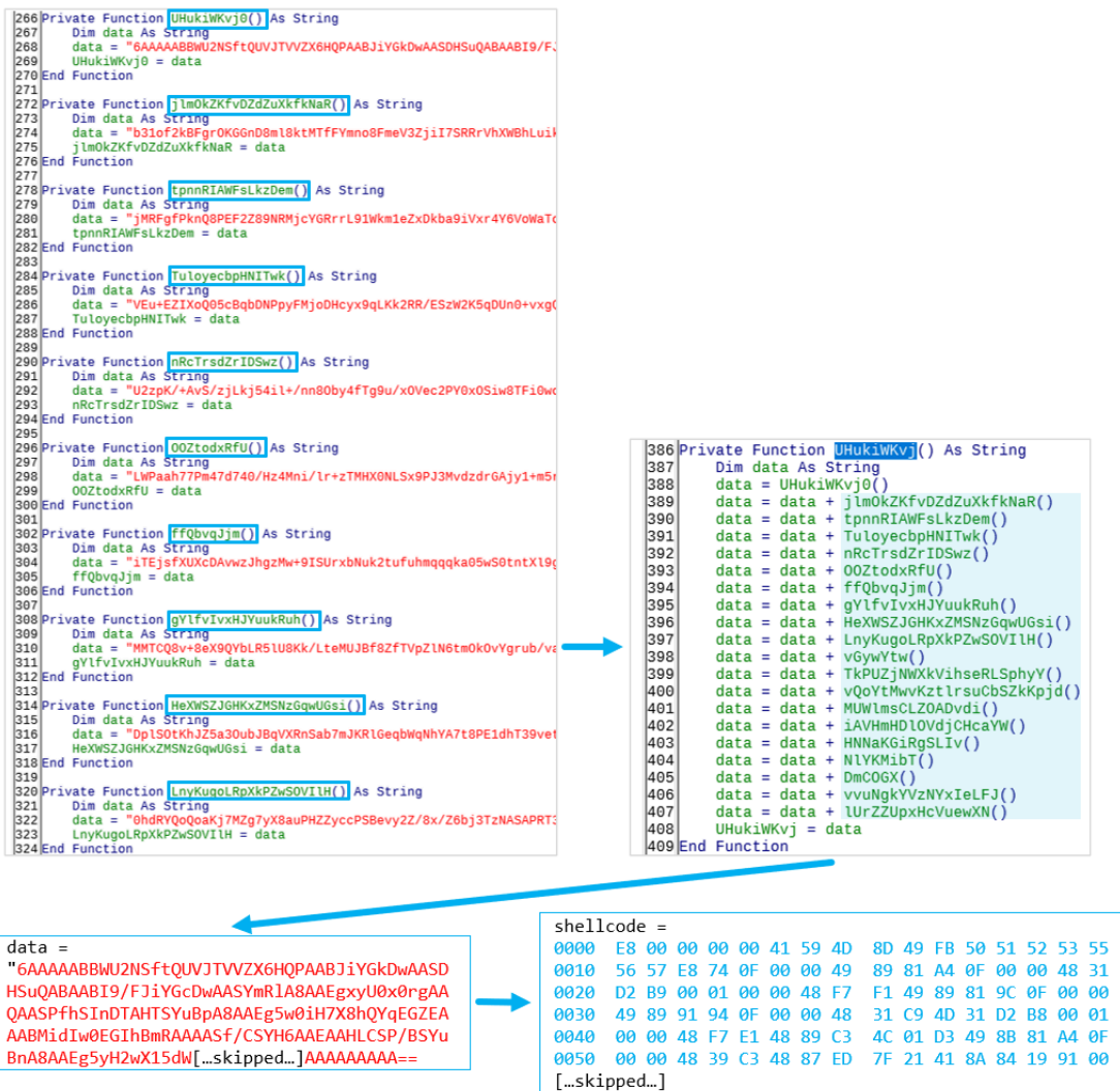
Figure 6. Reassemble the Base64-encoded and split Shellcode
