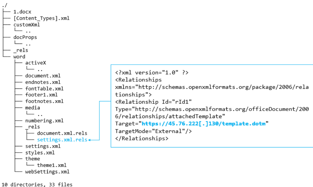
Figure 4. Word file's structure that uses Remote Template Injection
