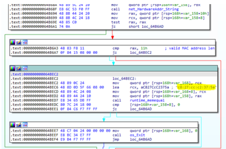
Figure 1. HardwareAddr.String() call, hardcoded MAC address, and os.Exit() call
