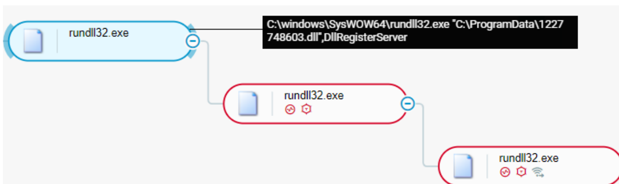
rundll32 executes Emotet: DllRegisterServer DLL entry point as seen in the Cybereason XDR Platform
