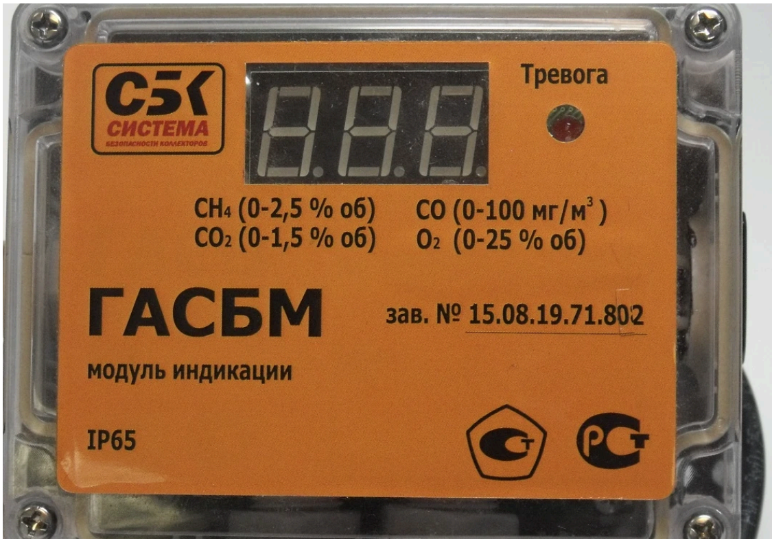
Gas analyzer of the security system (GASBM)
