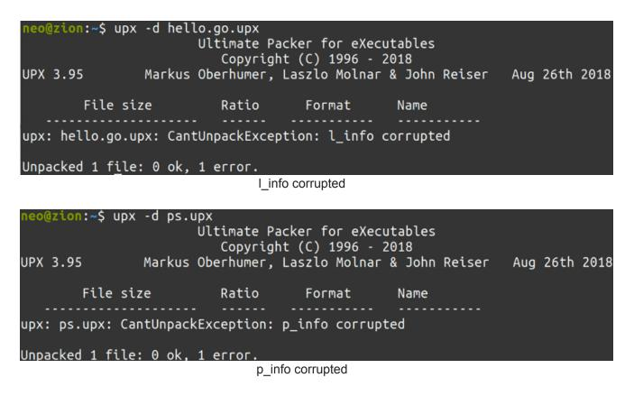
In order to understand what each of these corruption means, we need to dig further down and try to understand how the UPX header builds up after packing. We will find valuable information in the open source project's source code, inside <u>linux.h</u>:
