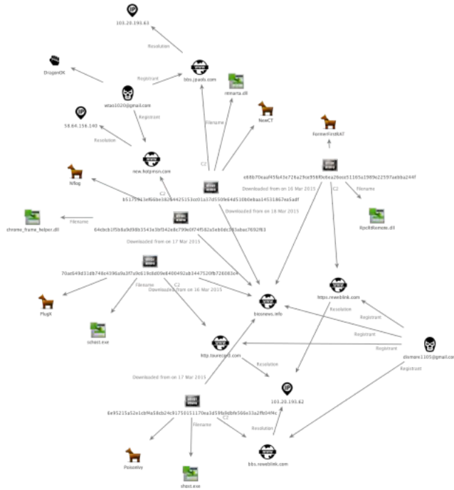
Figure 7. Relationship between five additional backdoors used by DragonOK and their C2 servers in this campaign.
