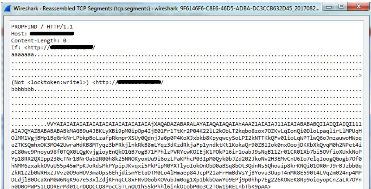
Figure5. Specifically crafted HTTP request with an encoded shellcode
