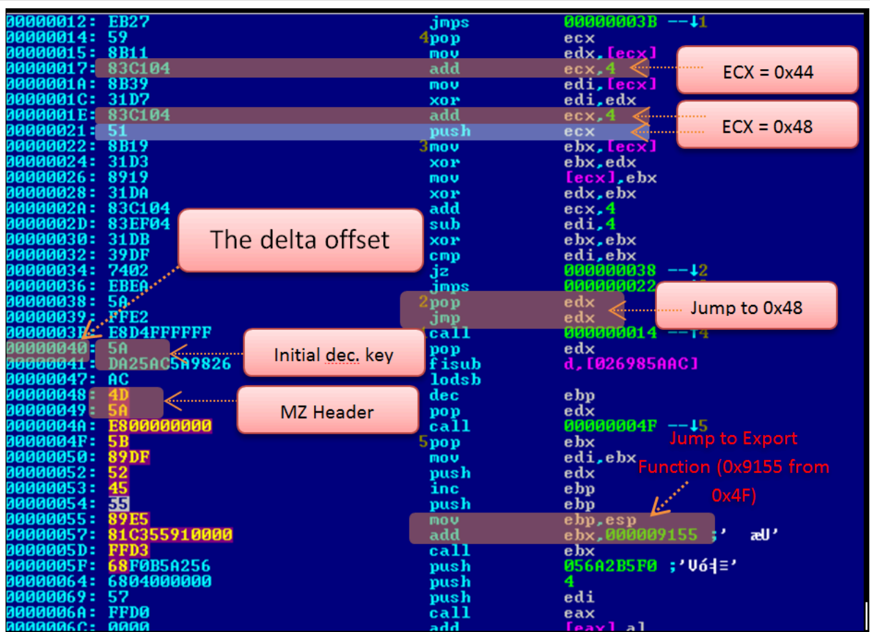
figure 5: the shellcode structure including the MZ header
