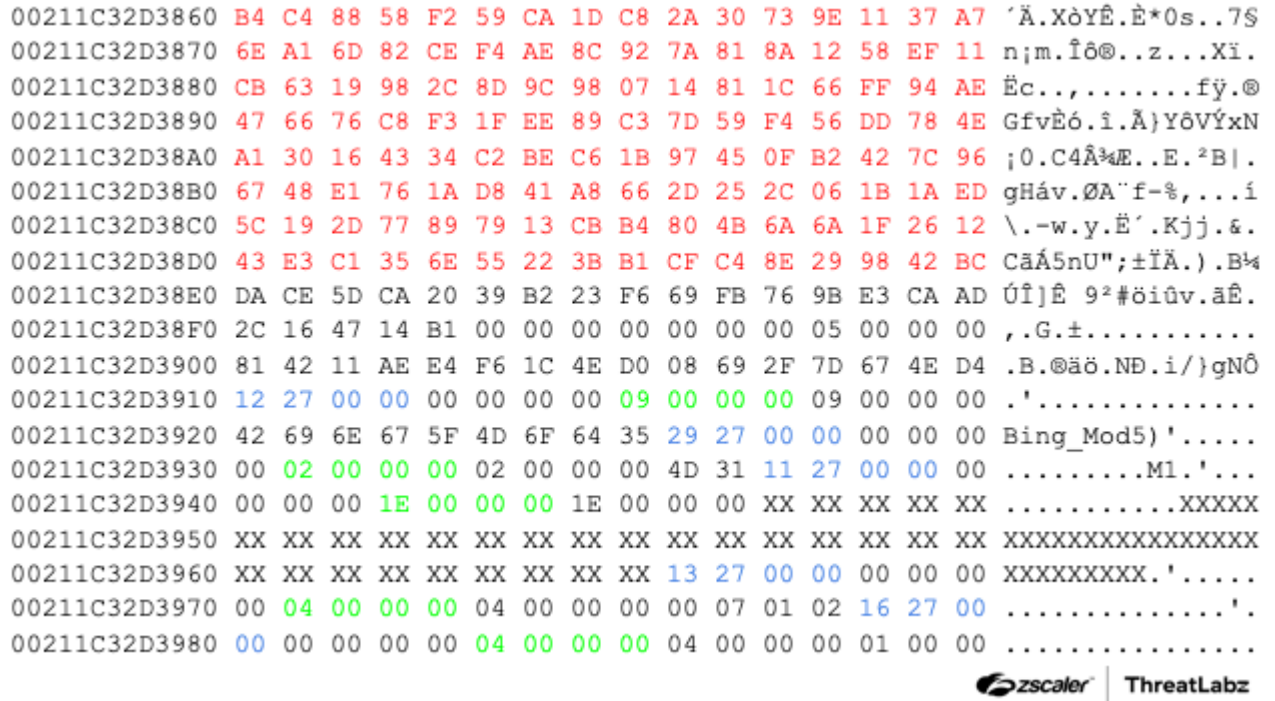
Figure 4. Zloader BinStorage object for a hello message (prior to encryption)
