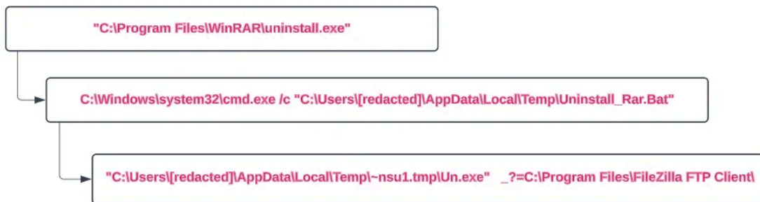
Figure 4: Process tree of uninstalling WinRAR
