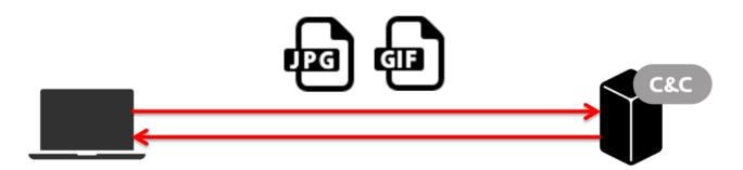
In case of the C&C server's unavailability, the backdoor component had yet another "backup solution" – a hardcoded URL pointing to a fake image (hosted on a free blog webpage) that contained the address of an alternative C&C server.
