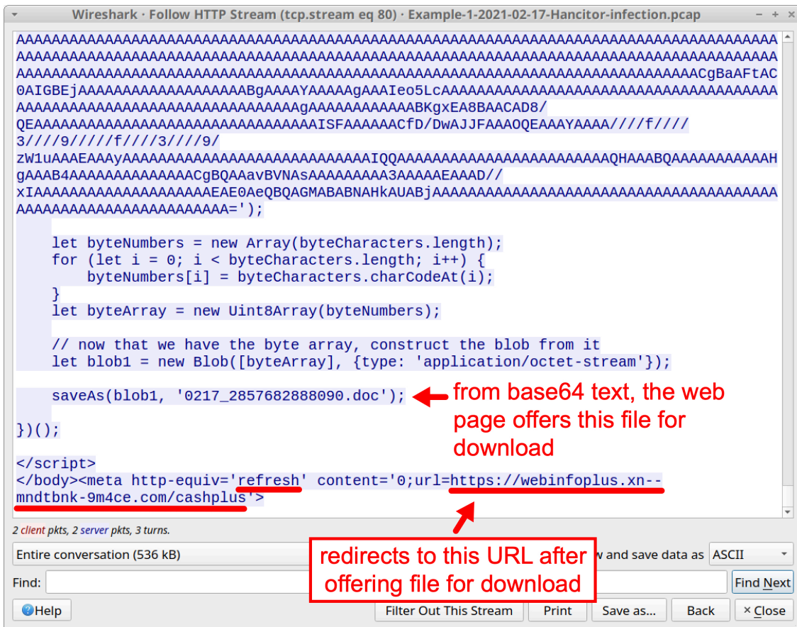
Figure 11. Script showing file name for the malicious Word document and refreshing the browser to a different URL.
