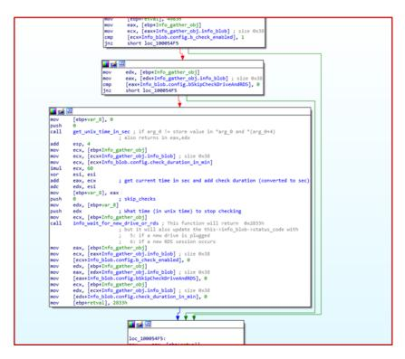
Triggering monitoring based on configuration
