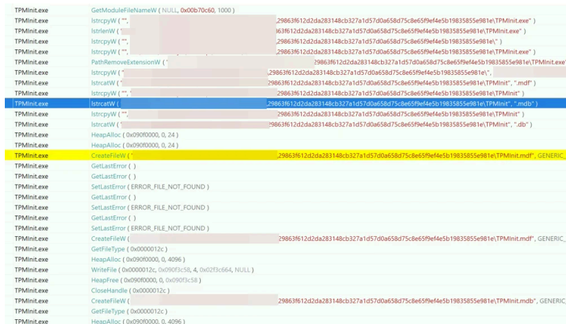
Figure 25: Analysis of TpmInit.exe, showing creation of TpmInit.mdf and TpmInit.mdb
