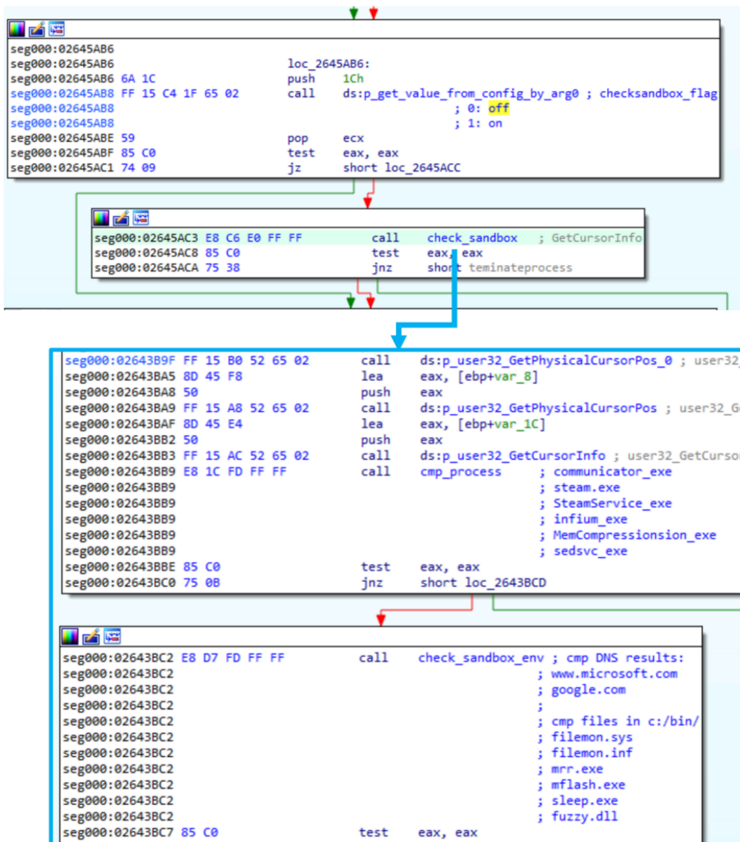
Figure 14. The anti-sandbox capabilities are enabled by the value of configuration.
