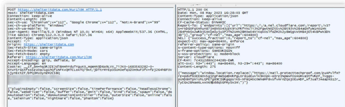
Figure 5. Content of POST request and server response using “Collect and Send User Data” JavaScript
