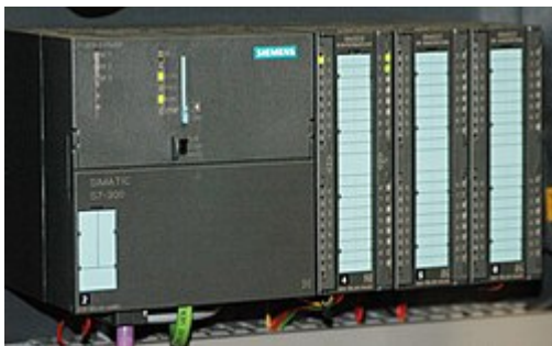
Siemens Simatic S7-300 PLC CPU with three I/O modules attached
