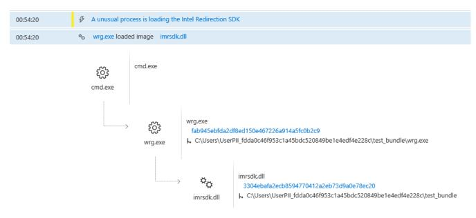
Figure 7. Windows Defender ATP detection of malicious AMT SOL channel activity
