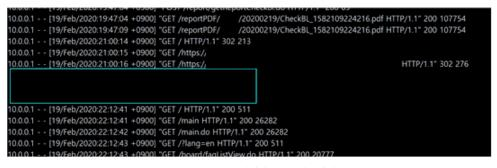
Figure 18: Traces of deleting of web logs.
