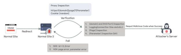
Figure 50: Proxy tool operation method.
