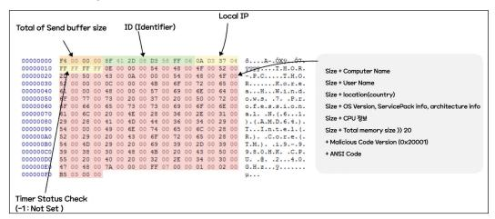
Figure 42: Data structure for sending information on infected devices.
