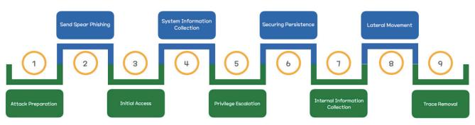
Figure 3: Overall attack process.
