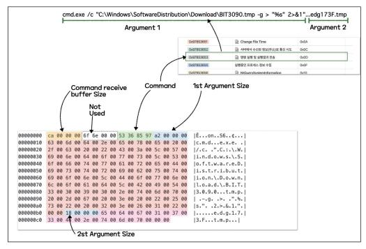
Figure 43: Data structure when sending commands.
