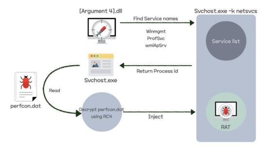
Figure 33: Detailed process of injector malware action.
