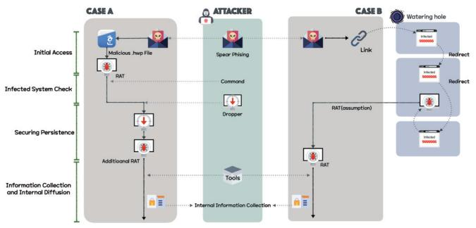
Figure 2: Two types of attacks using spear phishing.
