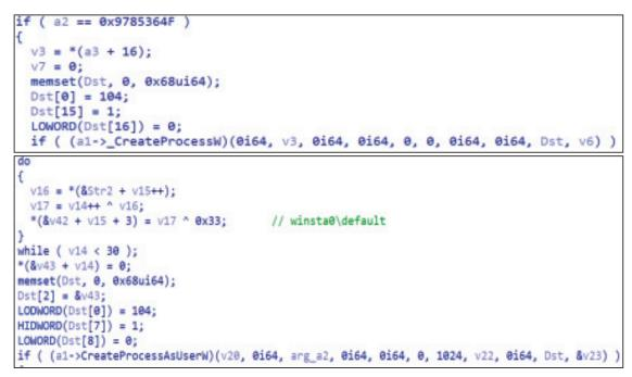
Figure 10: Additional processes are executed by calling the CreateProcessAsUserW and CreateProcessW functions.
