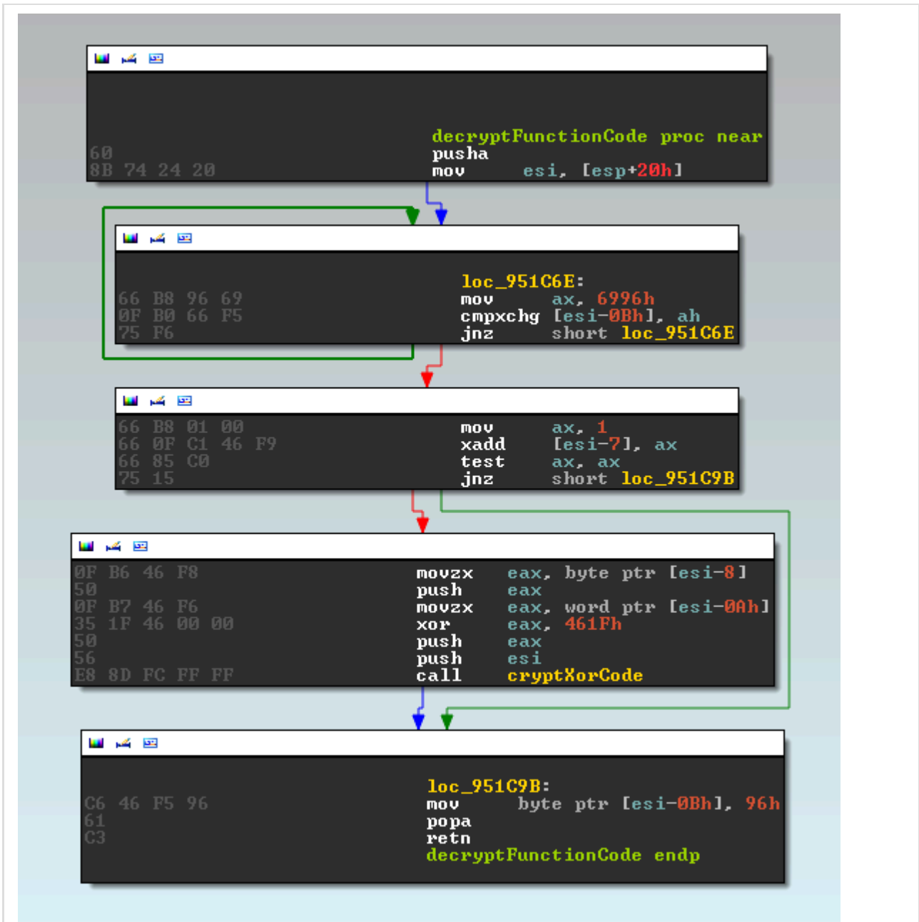
Fobber's on-demand decryption code for functions, revealing the parameter offsets necessary for decryption.
